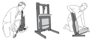
Fold out the two legs and twist them 3/4 of a turn, so that they are facing forward and the back section is stable.
