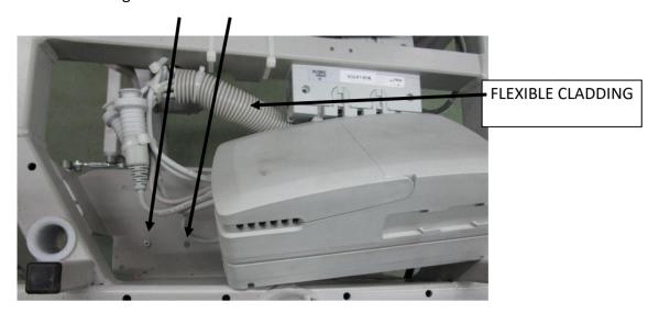
8. Using the cutting pliers, remove the ties securing the flexible cladding and remove the cladding.
