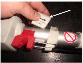
15. Drag the trigger lock in the notches.
