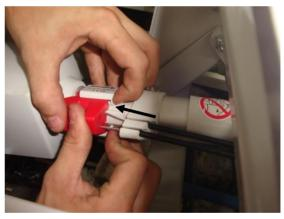
16. Drag cables support to spacer strip and screw it with the regular slotted screwdriver.
