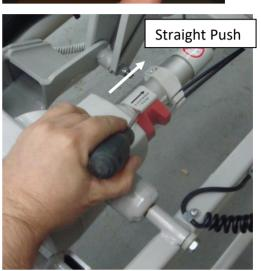
7. Remove the trigger lock, the trigger and the spacer strip.
