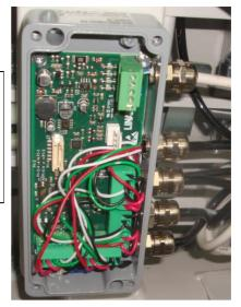
6. Unscrew all cable holder screws with a #3 small slotted screwdriver.
