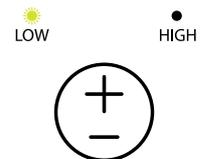
This function is used to silence the Audible Alert. The LED will remain lit if the Audible Alert has been silenced previously, however a fault is still detected. Refer to the power switch in order to re-set fully. If the Audible Alert continues to sound repeatedly, along with an illuminated light, then an engineer must be called.
