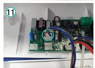
10. Connect Mercury Advance membrane 14 way header to the PCB, make sure that all pins of the header are connected.
