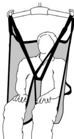
In the standard application the leg supports are crossed before they are hooked to the slingbar.
